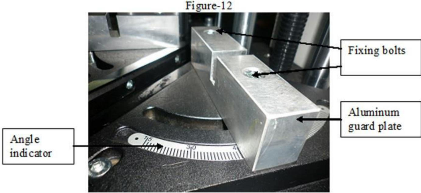
Switch the machine to single head mode. Slacken fixing bolts, set the front and rear aluminum guard plates at the desired angle on the angle indicator and the retighten the bolts. Perform the welding operation by using the buttons on the movable head. (Figure-12)
